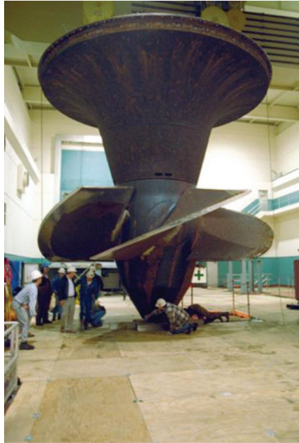
FIGURE 4.12 Kaplan turbine. (Images are courtesy of the U.S. Army Corps of Engineers, Louisville, KY.)
